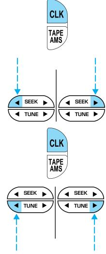
When in clock mode, the media information will display for 10 seconds, when the radio is turned on, and then revert to clock information. Anytime that the media is changed, (new radio station, etc.), the media information will again display for 10 seconds before reverting back to the clock. In media mode, the media information will always be displayed.
